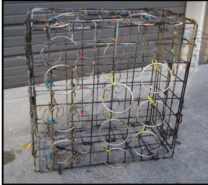
**Figure 8.** The back panel of pot number 1, with the rings. The rings with the cotton polyester cord have blue zip ties and are in the lower left quarter of the pot. All the natural cords have disintegrated and the color-coded zip ties show the original placement of the cords.
