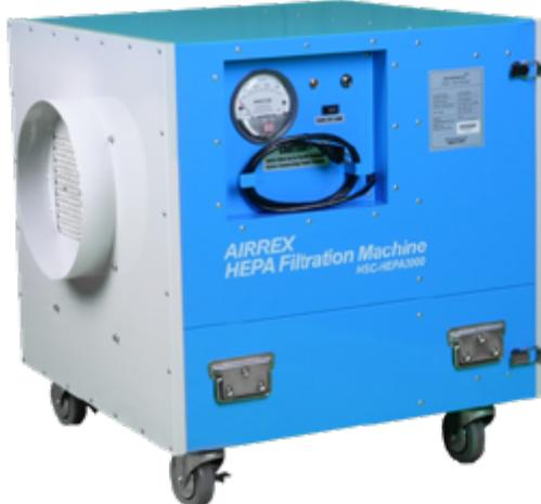
The AIRREX HSC-HEPA 2000 is a high efficiency particulate air filter that can remove at least 99.97% of airborne particles 0.3 micrometers in diameter. Particles of this size are the most difficult to filter and thus are the most penetrating particle size. Particles that are larger or smaller are filtered with even higher efficiency.
