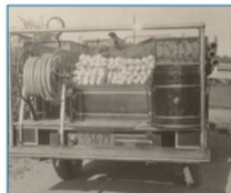
Rear view of new Moreland State fire truck May, 1930 assigned to Riverside County. Drinking water insulated container on the right. Back pump filling nozzle in platform at left. From the Fritz-Metcalf photographs collection.
