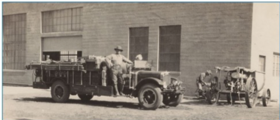
State Fire Truck on Moreland 2-ton chassis built in State Highway Shops 1929 at cost of $4200 ($76,000 in 2024 dollars), fully equipped. Tank 225 gallons of water, 105 gallon knapsack, pumps, 1000 ft. 1 1/2 in. hose, 500 ft. 1 in. base. Hand tools and kitchen equipment for 50 men. Top speed was 40 miles per hour. From the Fritz-Metcalf photographs collection.
