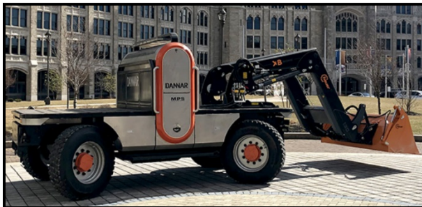
Mobile Power Station® Battery Platform, Semi/Fully Autonomous, DANNAR
