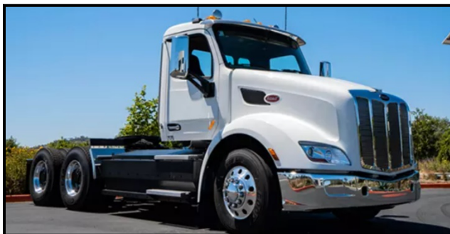
Class 8 Peterbilt 579 powered by a Meritor Blue Horizon 14Xe™ ePowertrain
