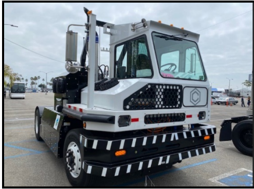
Hydrogen Electric Hybrid Yard Truck, Capacity Trucks
