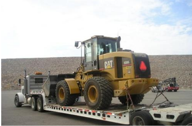
Fleet relocating a front-end loader using a heavy load trailer known as a "low-boy"
