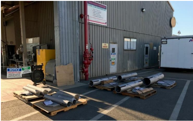
Pipe reinforcements fabricated by the La Verne Shops for the Perris Pumpback facility shutdown
