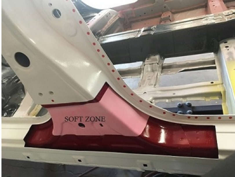
Pictured: Advanced technology steel module showing different ratings of steel, weld points, and floor reinforcements.
