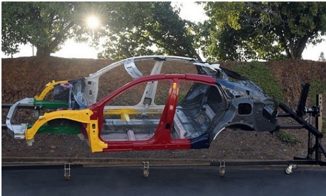
Pictured: Advanced technology module on a rotisserie-like device allowing the program representatives to learn appropriate repair techniques of the advanced vehicle safety technologies and engineering advances.
