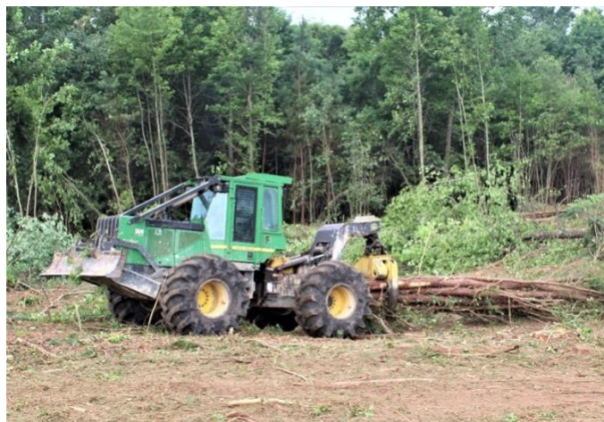
Figure 2. Grapple skidder pulling a pile of trees. Image credit: Patrick Hiesl, Clemson University.
