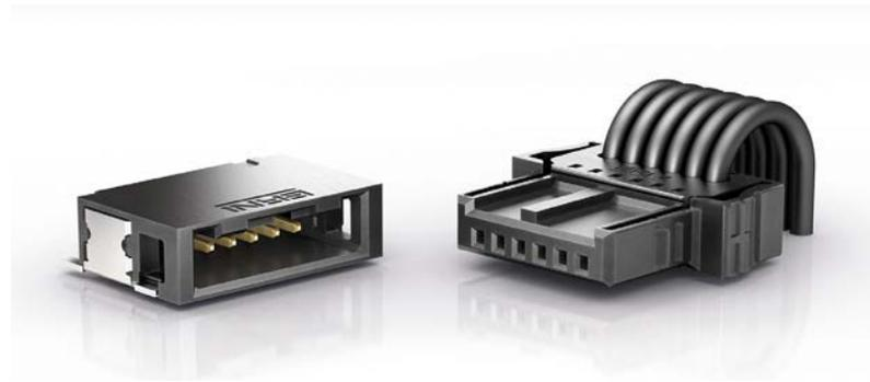
ERNI’s MicroBridge is available in straight and angled surface mount versions. The female connectors are available as insulation displacement connectors (IDCs). They are available with a 90° cable outlet. Pin counts are from two to 20. The connector conforms to US Council for Automotive Research (USCAR) and LV214 and also known as VW75174.
