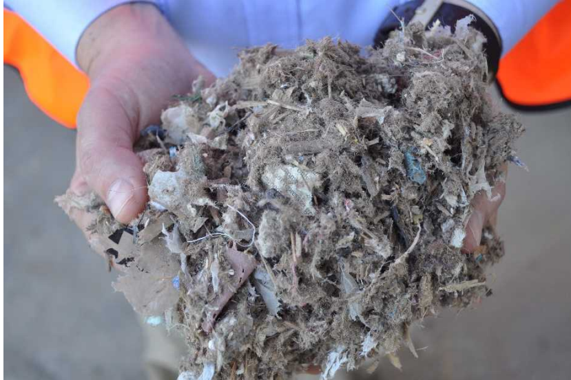
Figure 10. SUEZ-ResourceCo, Wingfield, sample of waste-derived, low calorific fuel destined for Adelaide Brighton Cement
