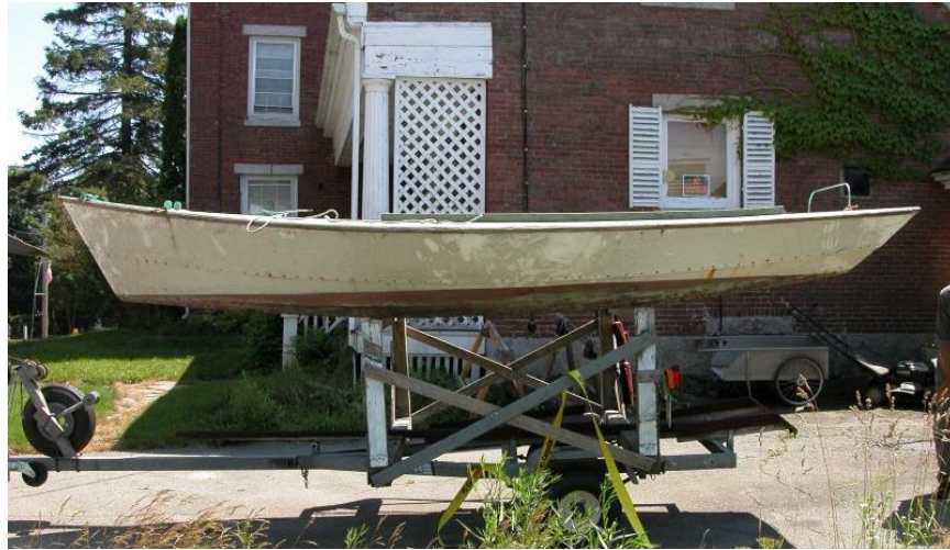
The Friendship catboat has a distinctive shape versus other catboats. The Friendship has a flat cross-planked bottom with slight rocker front to stern, two chines or boards per side, and a pronounced slanting bow stem and stern transom. Friendship catboat COTLEY, Gift of Elizabeth Toraason, 1998.27.
