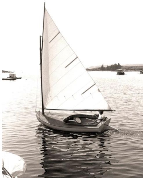
When most people think of catboats, they think of a Beetlecat, like the one pictured, with the blunt bow, broad beam, and barndoor rudder. The Friendship catboat is narrower with a slanted bow and transom. Maynard Bray Collection, LB2013.1.124.17.
