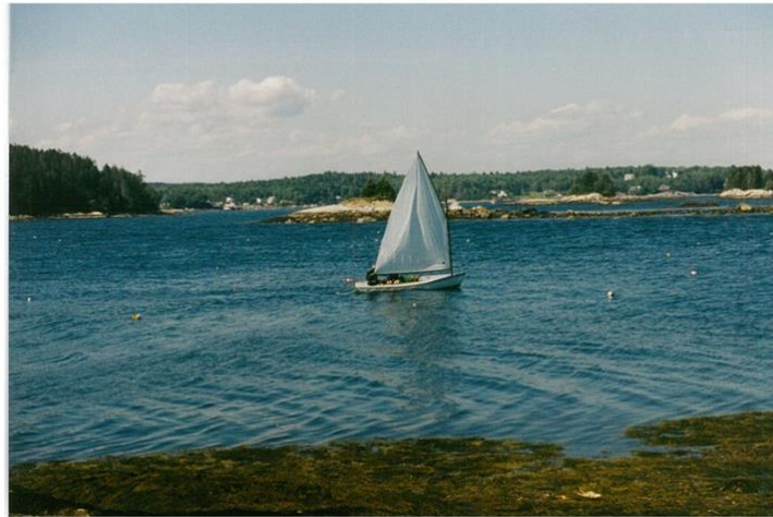
Friendship catboats, like COTLEY, were designed as light air boats to take advantage of Maine's light winds in island-sheltered harbors. Should the wind gust up, the sail could be reefed. Gift of Elizabeth Toraason, 1998.27.
