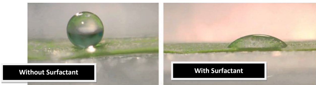
Figure 1. Comparison of water droplets on waxy leaf surface, with and without surfactant.
