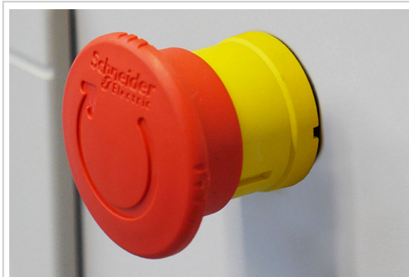
Fig. 31: Emergency stop switch - inactive
