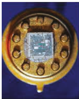
Figure 4. Analog Devices’ ADXL 50 is a monolithically integrated capacitive accelerometer with electronic functionalities, including an oscillator, demodulator, pre-amp, buffer amp and passives. It was primarily used for supplemental restraint systems (airbag) deployment. Credit: Analog Devices
