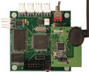
Fig. 3: The NARATA wireless node was developed for structural health monitoring applications. The node is 4 x 4 in. and contains an 8-bit embedded microcontroller, 128-kB flash memory, 128-kB RAM, four 16-bit ADC channels, two 12-bit DAC channels, and a power amplified IEEE802.15.4 radio. (Photo courtesy of University of Michigan WIMSS)
