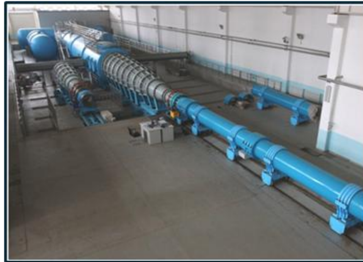
Figure 2 – CAS IOM JF-12 Shock Tunnel, Duplicating Hypersonic Flight Conditions at Mach 5 – Mach 9 111
