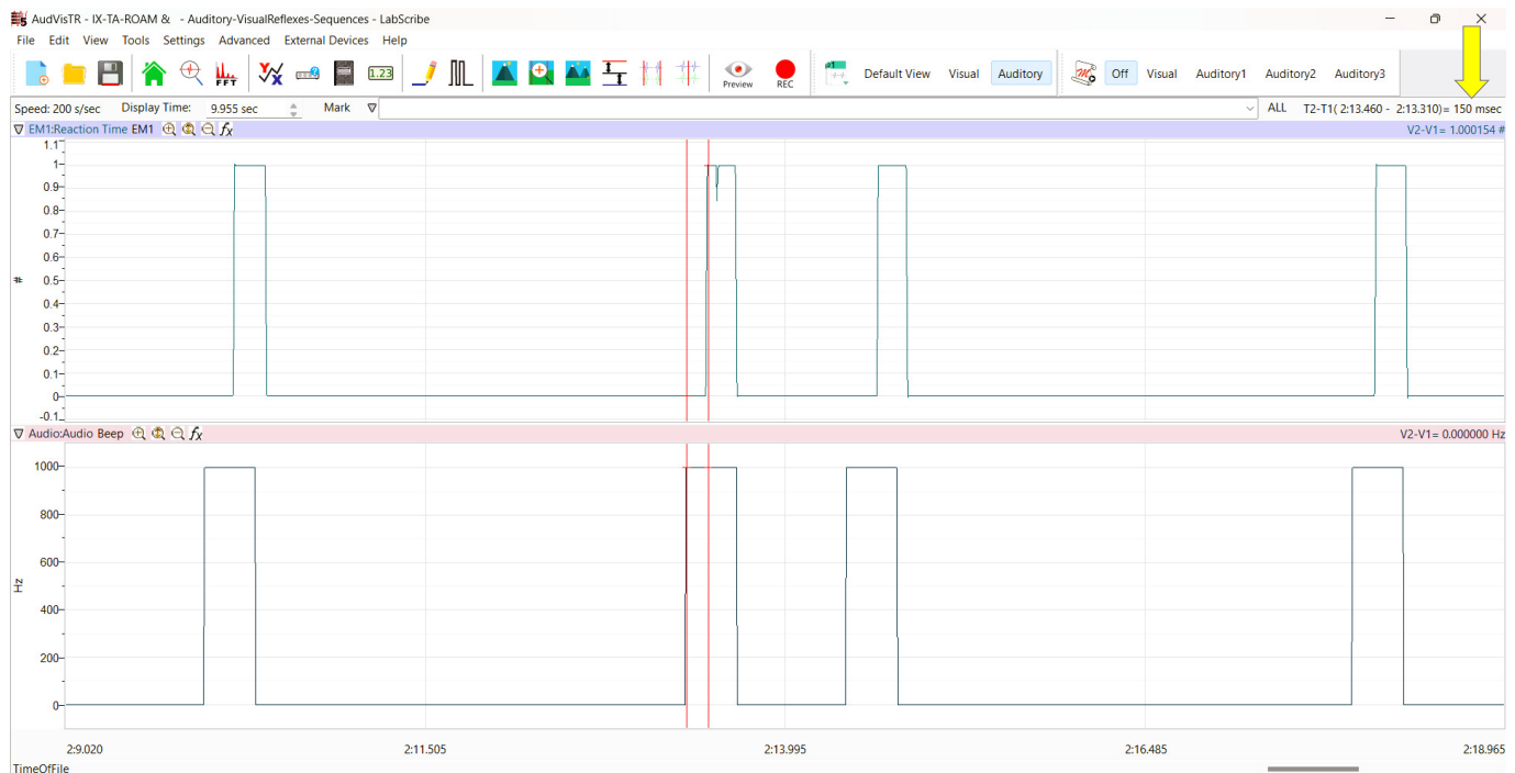
Figure HN-1A-L7: An auditory signal, followed by the subject's response. The two cursors are positioned at the beginning of the auditory signal and on the mark for measurement of the subject's reaction time ( T2-T1 ) in this trial = 150 msec.
