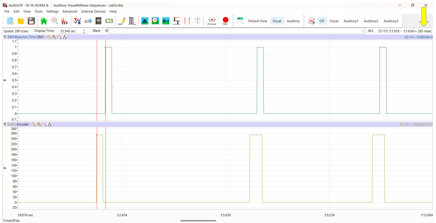
Figure HN-1A-L4: A visual signal, followed by the subject's response. The two cursors are positioned at the beginning of the visual signal and on the mark for measurement of the subject's reaction time ( T2-T1 ) in this trial = 285 msec.
