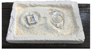
It makes a very safe, effective supporting material and heat has no effect on it. Of course, you could just break up some firebrick and put it in a crucible or other container, if you don't want to carve one from the brick. Where's the fun in that?
