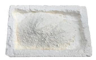
Smush and grind up the pieces to a powder-like consistency. The brick is very soft, and this is easy to do. Then pour what you have made back into the hollow of the brick. Now you have a great heat-
