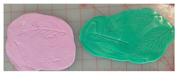
Castaldo makes crisper deeper images and can also withstand low melt metals (make lead castings) as well. These two molds seem to bear that out. The Green (Castaldo) mold is deeper and crisper. The purple (Cool Tools) may have set a little more quickly which adds to its failure to produce an equivalent image.
