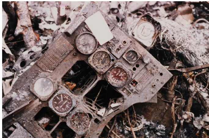
Figure 12 - Part of the Instrument Panel at the Crash Site (Transportation Safety Board Archives)
