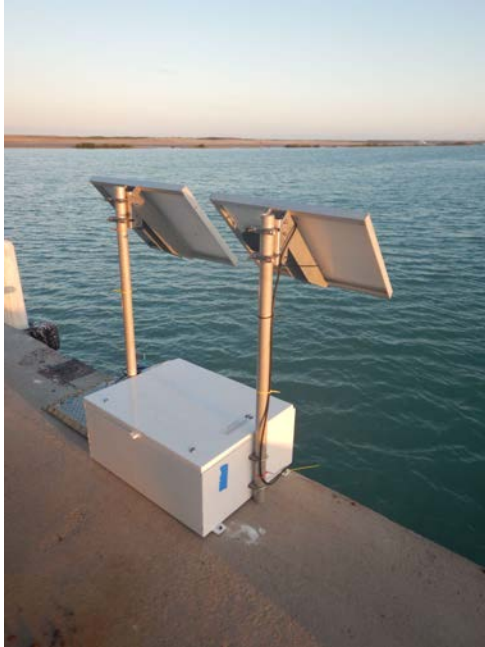
Horizontal mount ADCP - “Sidelooker” (13 stations)
