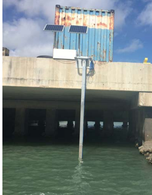
Horizontal mount ADCP - “Sidelooker” (13 stations)
