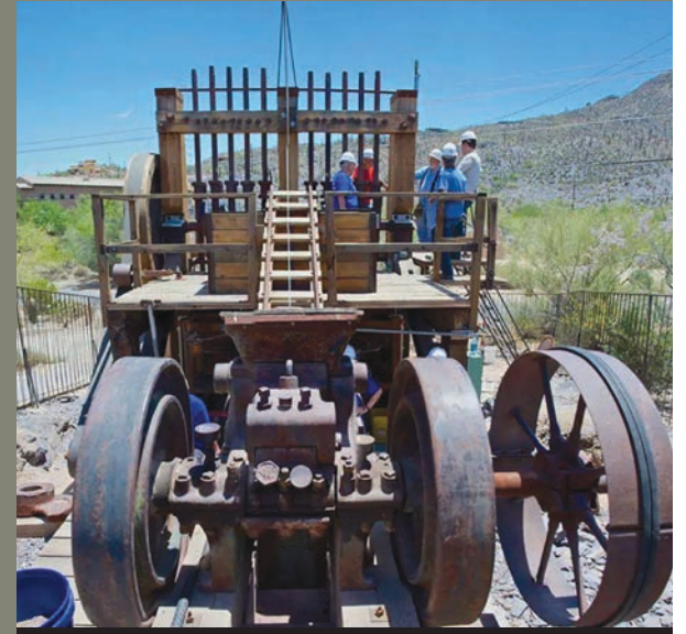
Arizona's only fully operational ten-stamp ore crushing mill. The ten 1,000-lb stamps slam down in synchronized motion to pound the ore removed from the mine into a fine gravel.
