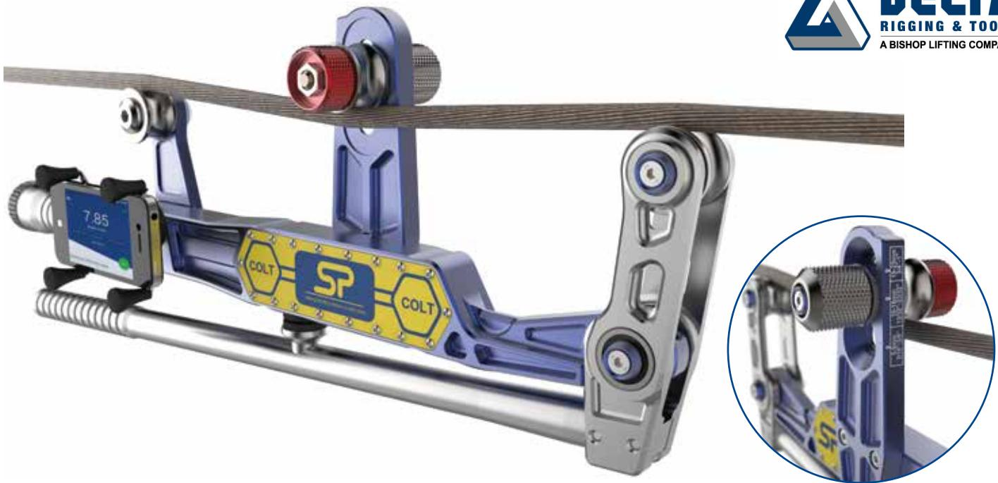
**The Straightpoint COLT is a lightweight tensionmeter for fast and accurate measurement of wire rope tensions up to 11,000lbf/5000 kgf and up to 1"/25mm diameter.**
