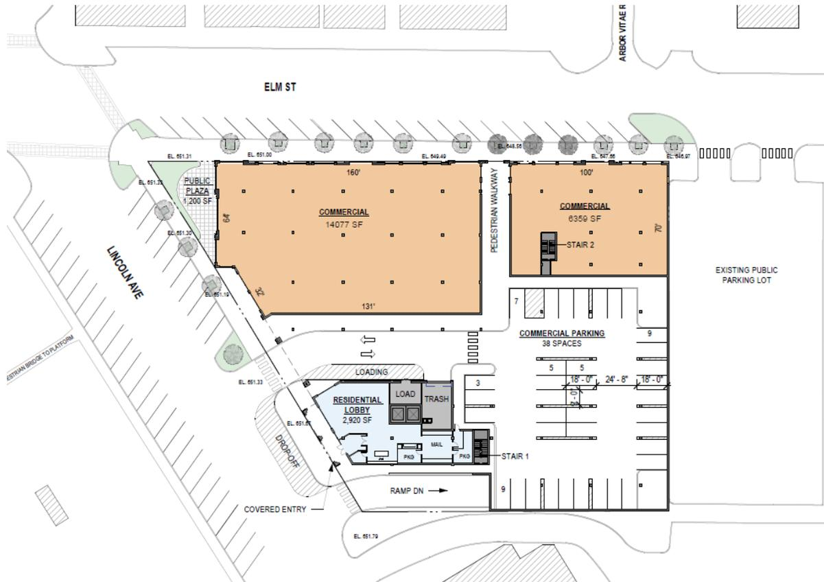
**Figure 5 – Current Concept Plan – Ground Floor Plan**
