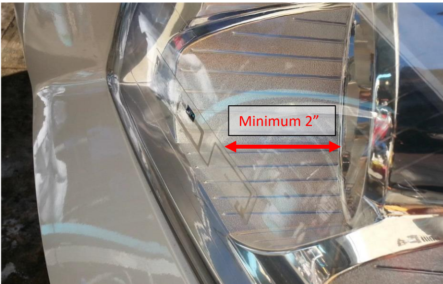
Side View to show Clearance for Distance between Headlamp Reflector Housing (above)
