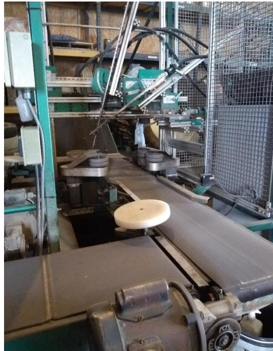
Efficient conveyor pruning method used at Overdevest Nursery.
