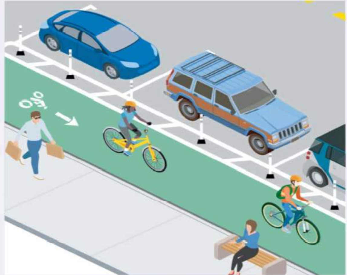
Figure 18. Parking-protected cycle track with narrow buffer and soft-hit posts obstructing the path of travel. A wheelchair user would not be able to unload from a vehicle in this design, and people using wheelchairs or walkers could not navigate safely down the buffer to an accessible crossing.
