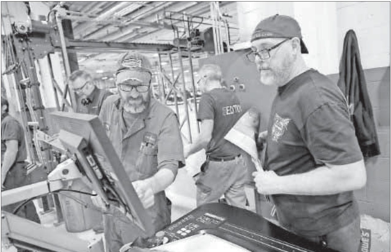
Jim Krassow and Darryl Carter adjust the ink levels while fine-tuning The Post and Courier's new printing press in North Charleston on Dec. 12.
