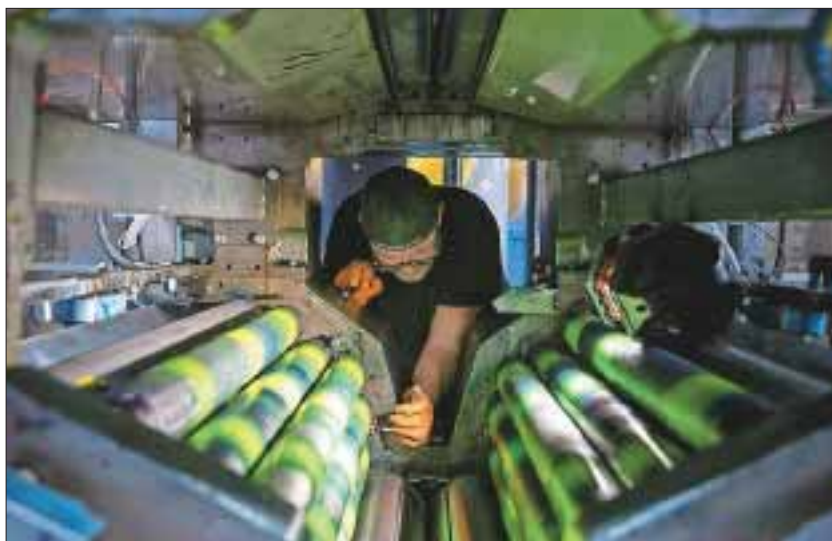
Darryl Carter squeezes between printing rollers to make adjustments to Evening Post Publishing's recently acquired 2008 Goss Magnum Single Width Press at a new facility in North Charleston.
