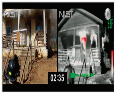
This image from a NIST experiment shows the difference between what we see with the naked eye (left) vs. a thermal imaging camera. The TIC clearly reveals heat at the front door.
