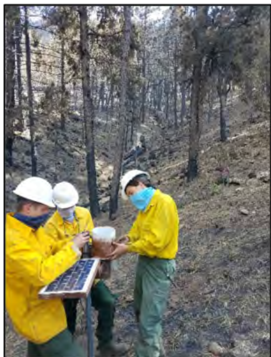
Figure 3. Installing the rain-triggered video camera in the age of COVID-19. View in the background is looking up the study channel. In photo, Luke McGuire (left), Francis Rengers (middle) and University of Arizona Geosciences grad student, Olivia Hoch (right).
