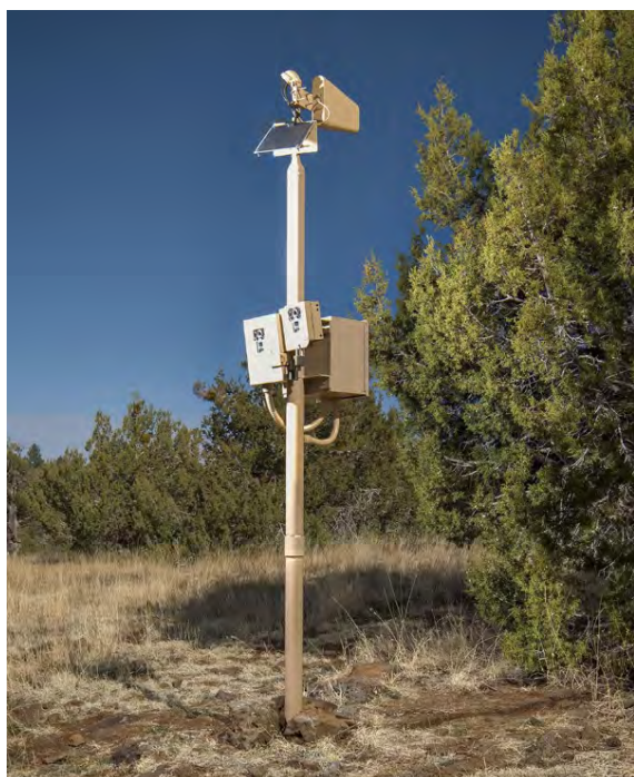
Figure 6. SRP has invested in innovative and proprietary LiDAR and field instrumentation, known as Flowtography, that provides real-time visual forest data.
