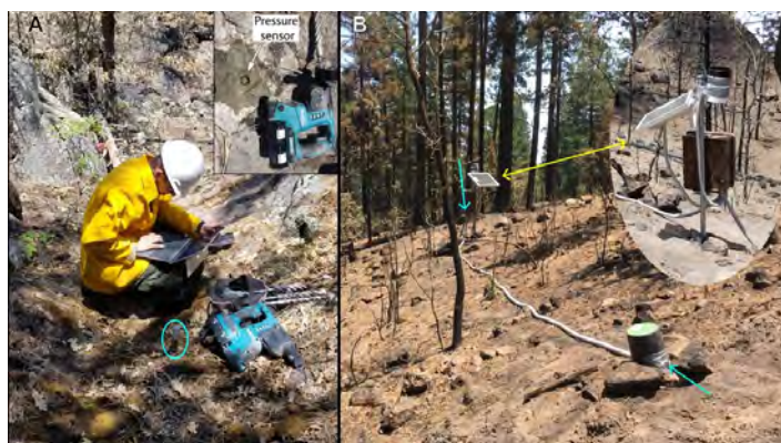
Figure 2. Panel A: installing a pressure transducer in a study channel. Luke McGuire is programming the pressure transducer (blue circle) before placing in the drilled hole. Inset photo shows a pressure transducer installed in the bedrock. Panel B: The USGS geophone setup. The inset photo shows the solar panel, rain gauge and battery and datalogger box. Two geophones (blue arrows) are attached to the datalogger via wiring through conduit. The datalogger starts recording when rainfall is above a programmed threshold.
