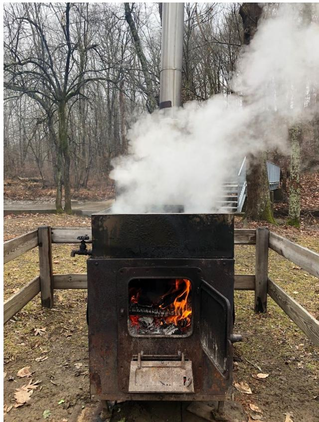
We will see how the evaporator uses fire to heat the sap and turn it into syrup.
