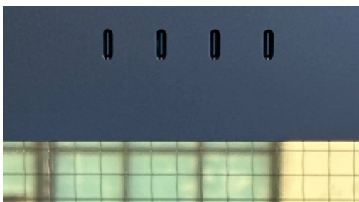
The ports on the M4 iMac are unlabeled but they're now all of the Thunderbolt 4 variety.
