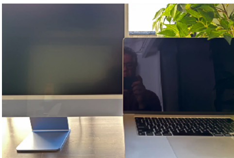
The new Nano-texture glass option (left) does a better job of diffusing glare and reflections than the standard glossy glass (shown on the MacBook Air, right). You can see how the Nano-texture glass diffuses the white wall behind me, while it is clearly shown over my shoulder on the glossy display.
