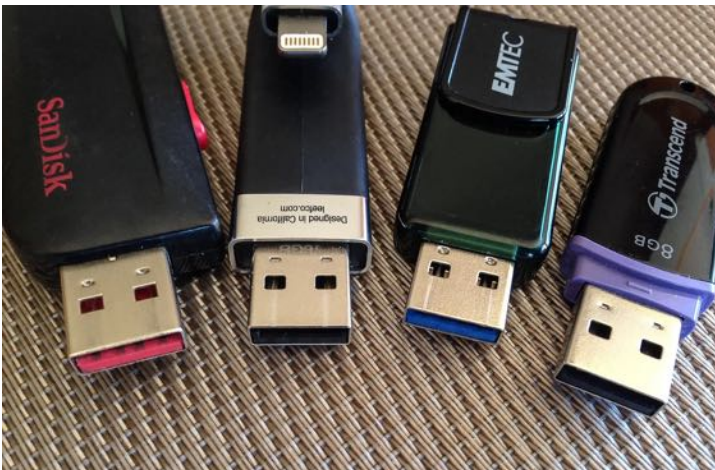
These USB-A flash drives need a USB-C adapter to be used on most modern Macs. Jacqueline Macou / Pixabay
