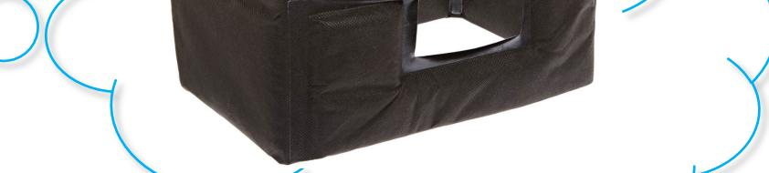
This is a **Thermal Wave Barrier**; it helps reflect engine heat away from the battery to ensure the anticipated life expectancy from the battery. **If you see a thermal wave barrier on the old battery, it is important to transfer it over to the new battery you are installing.**
