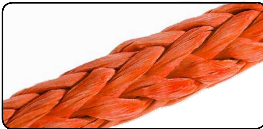
X-Trema Line is a twelve-strand, high-modulus polyethylene rope made from authentic Dyneema® fibers. Our X-Trema Line has an unmatched strength-to-weight ratio. Compared to a steel wire rope of the same size, it will match the breaking strength at only 15% of the weight.
