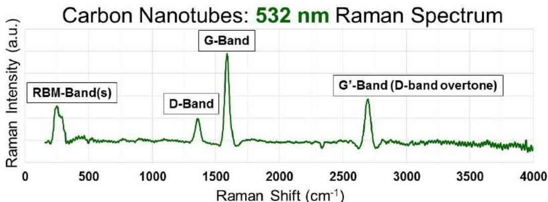
**Figure 2.** 532 nm Raman spectra of carbon nanotubes (CNTs), measured using BioTools' **Ramtest™-NANO** instrument based on **Ram-532™** spectrometer. This spectrum contains all important CNT Raman bands, which can be used for CNT characterization (please see text for detail).
