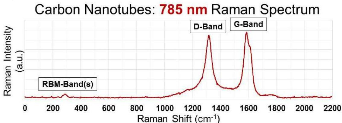
**Figure 3.** 785 nm Raman spectra of carbon nanotubes measured using BioTools' **Mobile μRaman™** instrument based on **Ram-785™** spectrometer in its high resolution configuration. **NOTE:** Extended range configuration of Ram-785™ recommended to include G' band of CNTs (please see text for detail).
