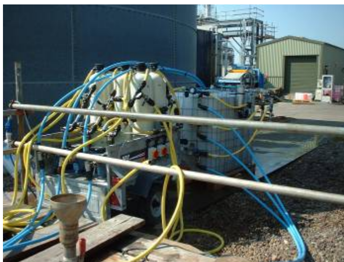
Figure 1. Set up of pilot two-stage filter rig at Hartleys
