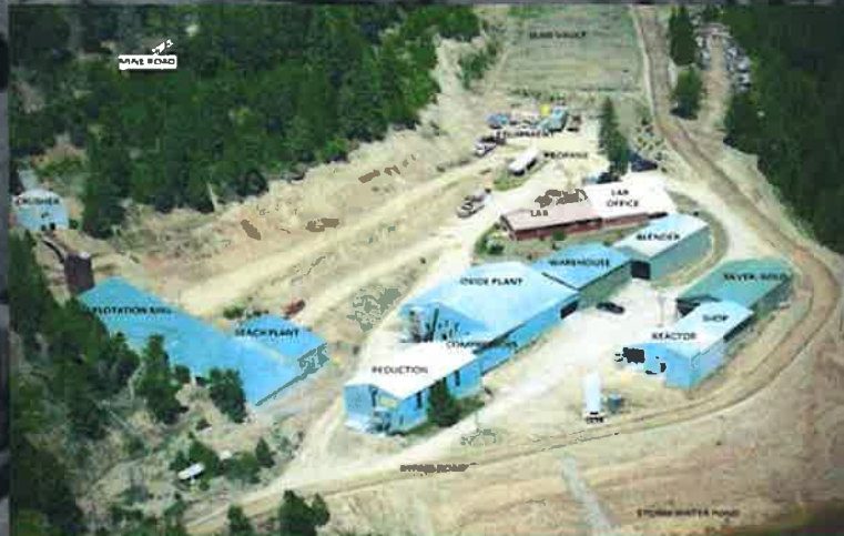
ANTIMONY SMELTER PLANT - THOMPSON FALLS, MONTANA NOTE: SMELTER CAPACITY EXPANDING TO 300 TONS PER MONTH OR 11 TONS PER DAY
