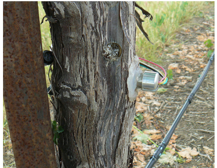
Installed FloraPulse sensor in a vine trunk at a UCD field trial. Photo: Ted Rieger
