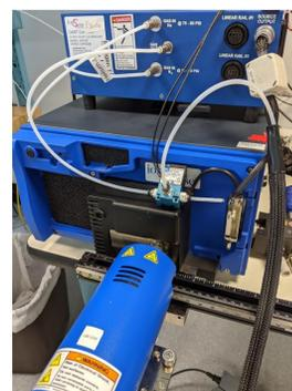
Figure 1: Pulse DART setup with solenoid shutter.
