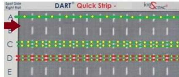
Figure 2: Schemes for sample movement through ionization region and ionizing gas sequence for continuous and pulse DART operation.
