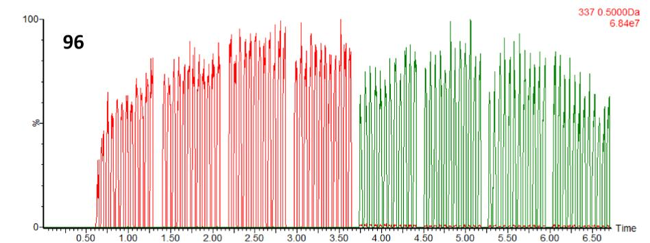
Figure 4: Representative EIC of codeine and fentanyl analyzed in a 96-sample array with pulse DART. Peaks for two rows are shown.
