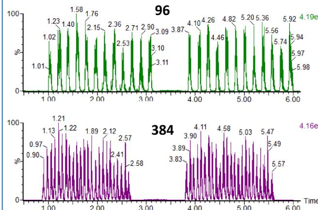
Figure 3: Representative EIC of codeine analyzed in a 96- and 384-sample array. Peaks for two rows are shown.
