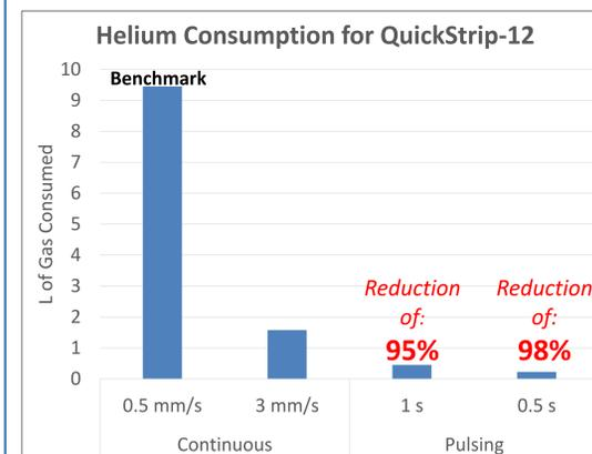
Figure 2: Helium reduction with pulse flow approach for DART compared to a continuous flow of gas.
