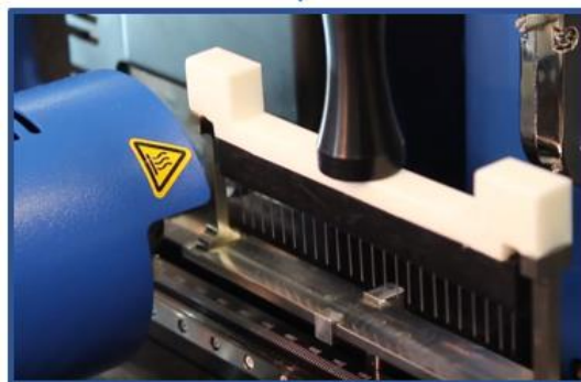
Fig 1: Direct sampling of beef followed by introduction to DART-MS of the 24-Pin Sampler via the automated linear rail
