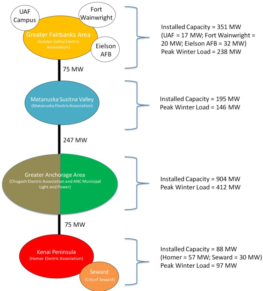
Schematic of Alaska's Railbelt Electric Grid, and the six utilities that share it. Note the Fairbanks area has three connected but separately managed electric grids that connect to the GVEA system. Bradley Lake and the Eklutna hydroelectric projects are not included in installed capacity figures because they are jointly owned assets.
