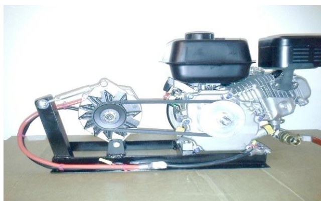
6.5 hp motor powered by wood/producer gas, which runs the 12VDC alternator/charger (Source: Mike Leister)
