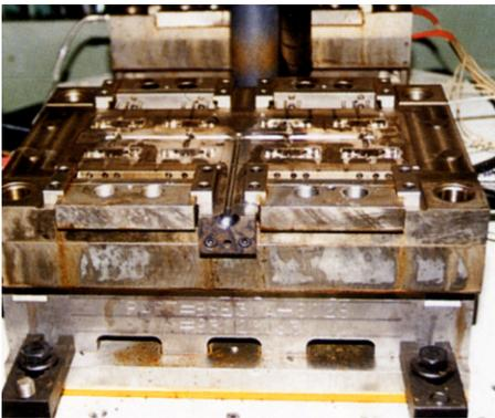
▲ Pyropel insulation ensures optimum temperature and flow conditions for exotic engineering grade polymers in hot runner injection molding.
