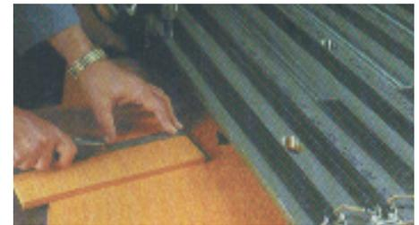
Pyropel is easy to use and requires no special tools. It handles like wood or any free-machining plastic. Pyropel can be drilled, milled, routed, and sawed using standard wood or metalworking tools.
