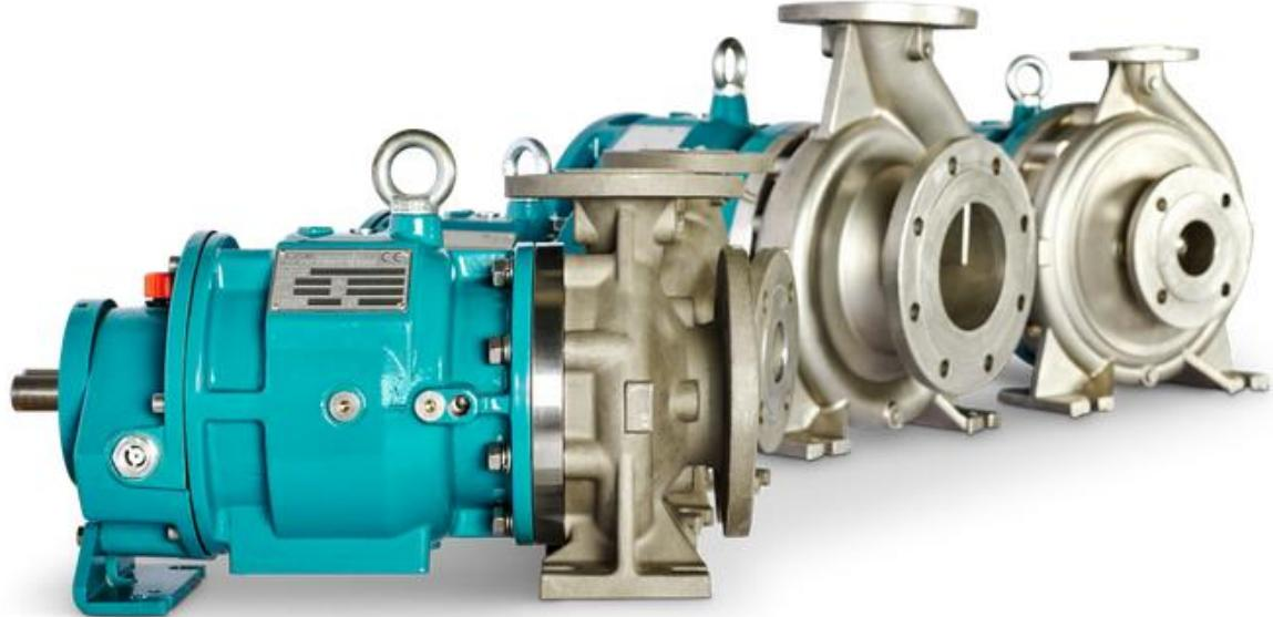
These little beauties (sad but true, in the pump world these are good looking!) are magnetic coupled pumps, so no mechanical seals to fail and leak. That's good isn't it?
