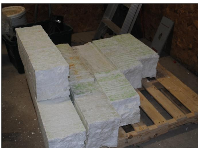
LEFT: Once the foam polystyrene is broken up, compressed and extruded through the machine, blocks are loaded onto pallets to be shipped to companies who use it to make consumer products.
