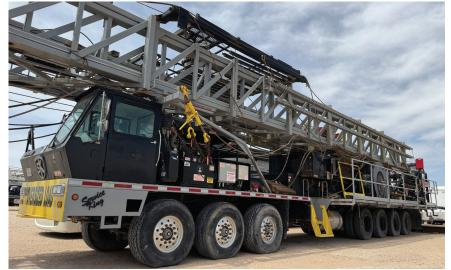
**VENTURE TECH XK-90 Power Swivel p/b** CAT C7.1 Tier 4 Diesel, HPU, Hoses, Remote Controls, Mtd on T/A GN Trailer
