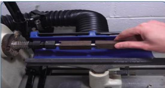
Mount the pen blank pieces and the lathe components onto the lathe.
