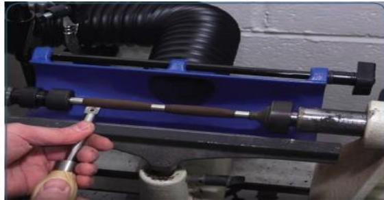
Turn the pen blank to the desired shape. The outside diameter of each blank piece should match the diameter of the bushings.
