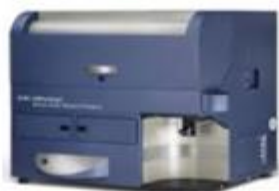
BD LSRFortessa X20 (5 Laser, 18 channels)
