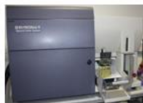
BD FACS Aria II (4 lasers, 18 channels)
