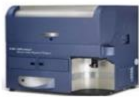
BD LSRFortessa (5 Laser, 18 channels)
