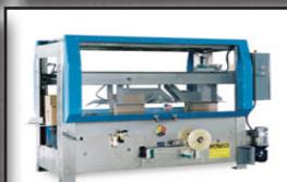
Our range of case erectors and sealers meets all needs from small, low volume applications to the most demanding high volume lines. From basic RCS and HSC cases to difficult doublewall heavy duty designs, we have a machine that fits the need. Closures are available in either hot melt glue or pressure sensitive tape.
